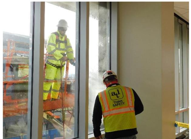
The ASTM E1105 test method determines if water penetration exists through an installed fenestration product. Similar to the test procedure used in ASTM E783, a specified pressure differential is established on opposing sides of the test specimen and the specimen is subjected to a uniform water spray for 15 minutes. The specimen is continuously observed for signs of water penetration throughout the duration of the test period.
