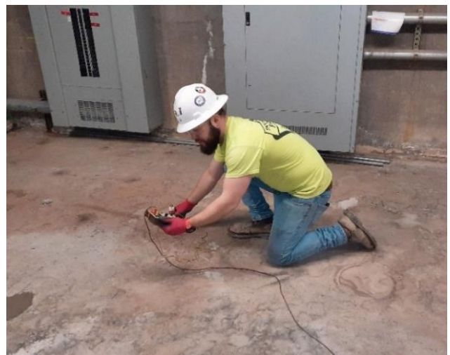
Upper: Ultrasonic Pulse Velocity testing (ASTM C597) Lower: Half-cell corrosion potential survey (ASTM C876)
