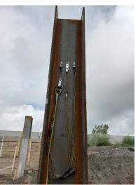
• Testing set up is quick and several piles can be tested on a project in a relatively short time period, making dynamic testing economical
