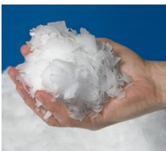
Ice flakes are often used to control concrete mix temperatures during the summer months.
