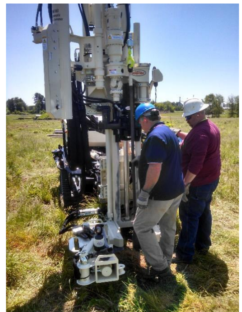
Soil Sampling with ATL Geoprobe Model 7822DT.
