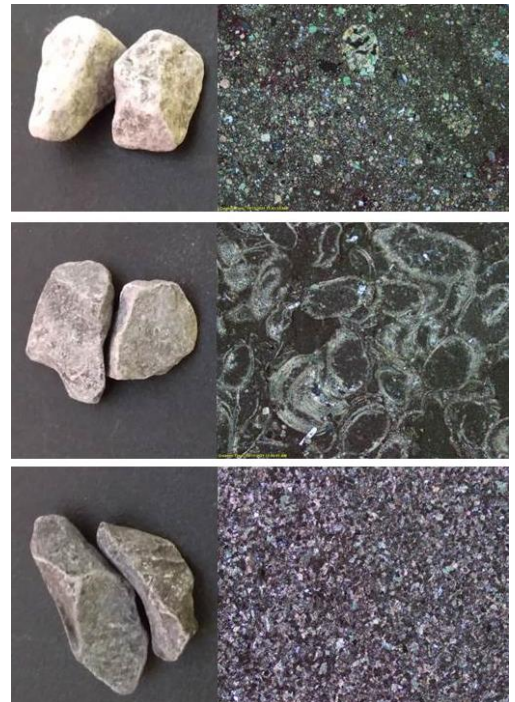
Macroscopic (left) and associated microscopic (right) views of concrete aggregates.
